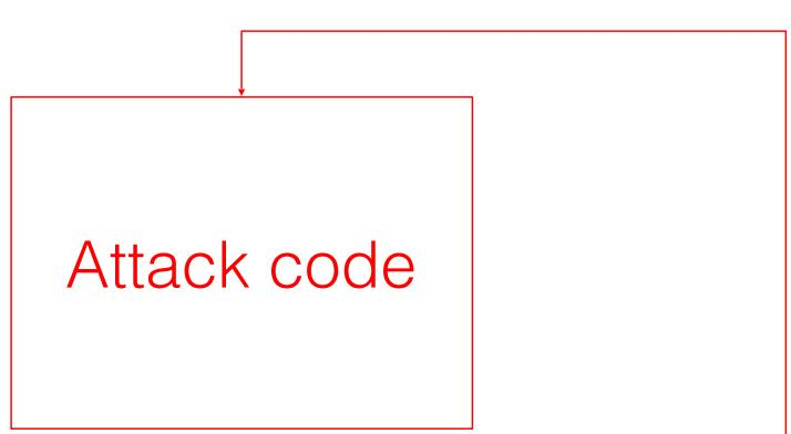
Change the return address to point to the attack code. After the function returns, control is transferred to the attack code.
