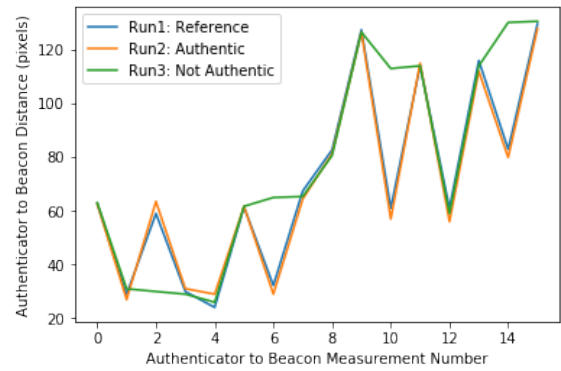
Fig. 14: Experimental results for FLATS design integrated into the ISCAS 85 benchmark c432. Registration, successful verification, and tamper detection events are shown.
